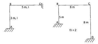
8. Develop the displacement transformation matrix for the structures shown in Fig. and hence derive the stiffness matrix. Assume EI constant for all the members.
