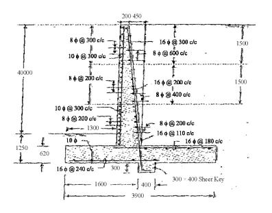
details of soil are safety bearing capacity 170 kN/m<sup>2</sup>, angle of repose 30°, unit weight of soil 18 kN/m<sup>3</sup> and coefficient of friction with concrete 0.45. Check the stability of the retaining wall.
