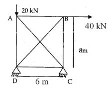
5. Analyse the following frame by displacement method if the support C sinks by 1000/EI in vertical direction.20
