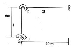
4. Analyse the following truss by flexibility approach.20
