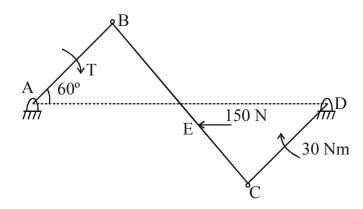
AB = 200 mm, BC = 700 mm, CD = 400 mmBE = 400 mm, AD = 700 mm.
